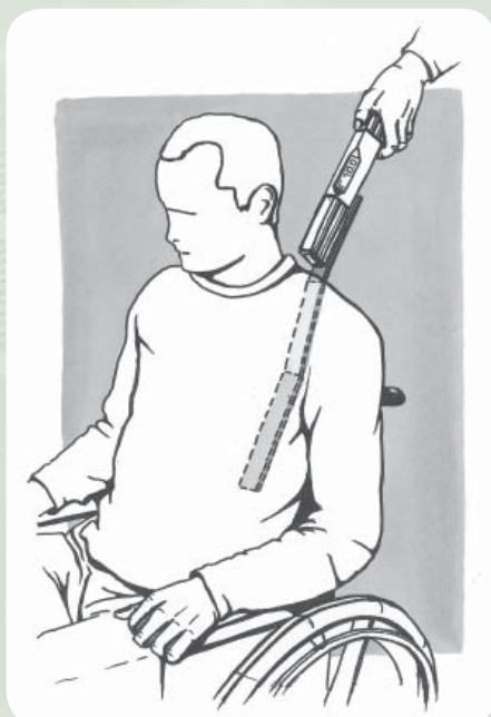
Figure 5: Measuring the functional backrest inclination
