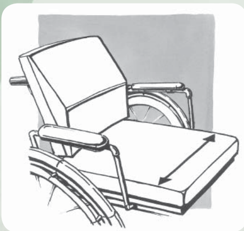
Figure 8: Measuring the width of the seat cushion
